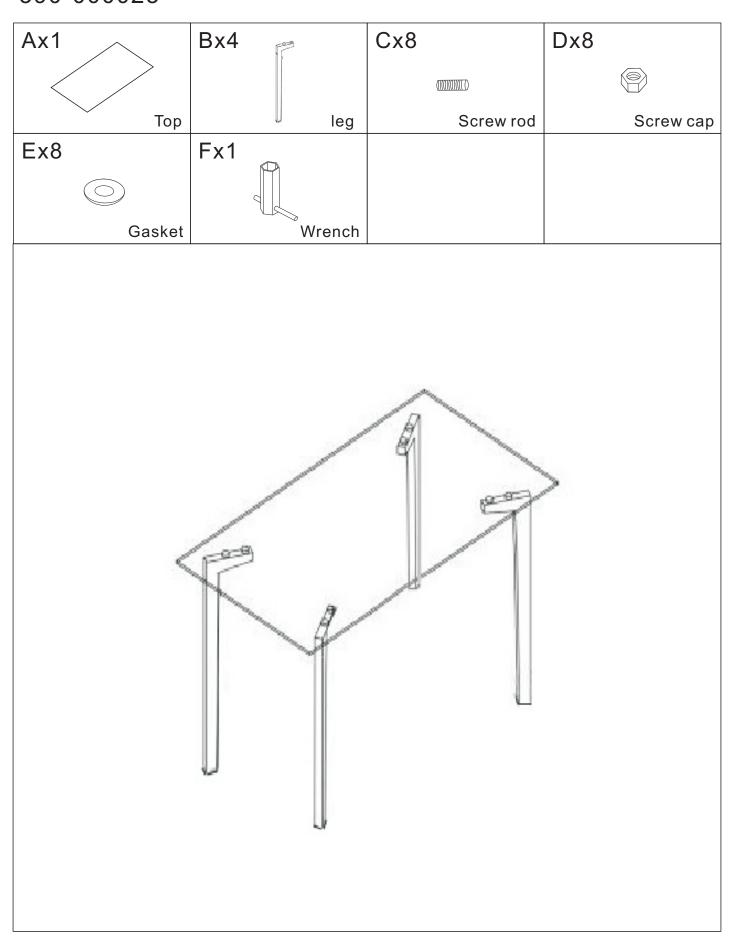
STEP 1: To put screws rod C and legs B on the top A firstly To fix gasket E and screw cap D with wrench F
