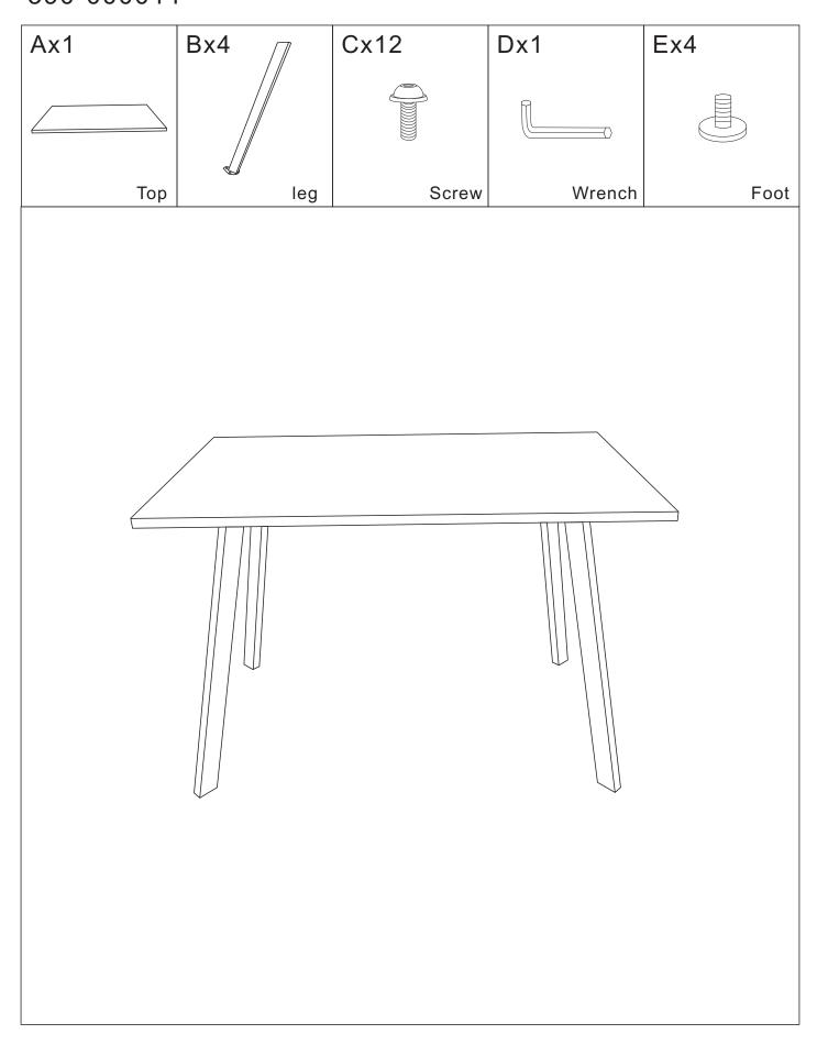
STEP 1: To put legs B on the top A firstly To fix screws C with Wrench D To fix foots E
