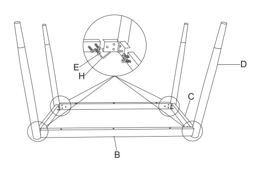
STEP 2: To put all the legs on the top A firstly To fix Gasket G and Screw F with Wrench H To fix foot I
