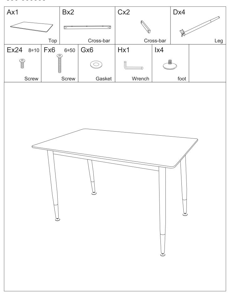
STEP 1: To fix Cross-bar B, Cross-bar C and legs D firstly To fix screws E with Wrench H
