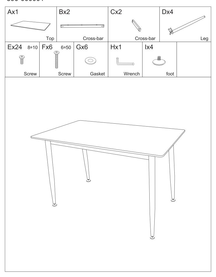
STEP 1: To fix Cross-bar B, Cross-bar C and legs D firstly
