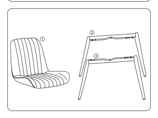
Please half tighten all the screws into the screw hole first. After All the screws are set in holes, fully tighten them.
