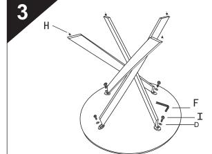
When tightening the Bolts, tighten sequentially. Do not tighten any screw fully and then towards the next one, this would cause the leg to misplace.
