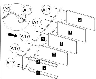
STEP 2 Join panel no. 1 to the unit by using Crosshead Screw m6.3 x 40mm (A17). Use Allen Key (N1) to tighten the Crosshead Screw m6.3 x 40mm (A17).
