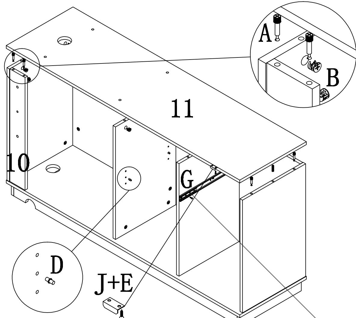
To put the shelves fix screw (D) inside,fix the lock metal minifix(J)
