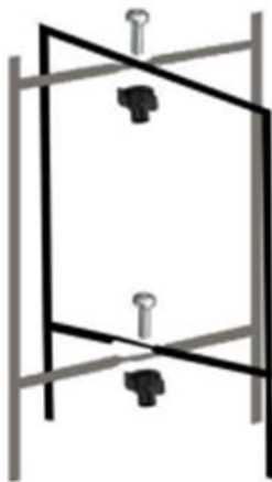
Screw on so that the plastic nuts stay on the bottom as shown in the image
