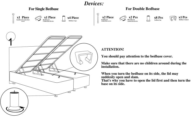
When installing the bedbase legs, you need to pierce the fabric under the bedbase at the level of the holes on the metal profile.
