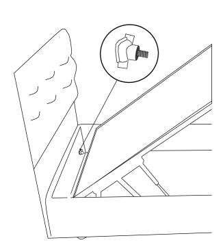
Mark the connection points of your bedbase or cot on the header with the help of a pencil. drill the head through the marked points and fix it in place with mounting screws.
