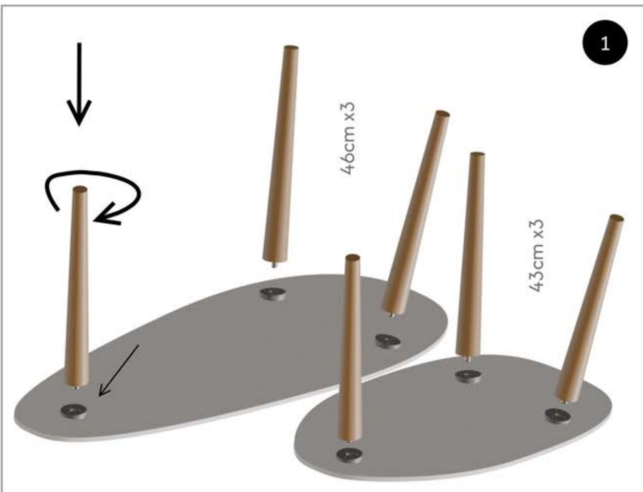
Attach the three 43 cm wooden legs to the 45x77 cm table by turning them clockwise until firmly secured. Repeat the same process with the 46 cm legs for the 46x116 cm table.
