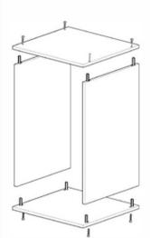
STEP 2 ASSEMBLE PARTS 3 & 4 WITH THE TREENAILS AND 4.50 SCREWS THEN ASSEMBLE PARTS 3 & 4 TO PART NUMBER 2 WITH THE
