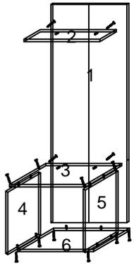
THE SIDE SURFACES ARE ASSEMBLED TO THE TOP AND LOWER SURFACES.
