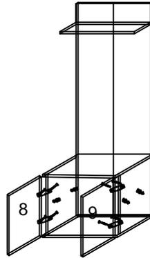
CABINET DOORS ARE ASSEMBLED TO SIDE FACES WITH HINGES. THE SHELF HOLDERS ARE ASSEMBLED.
