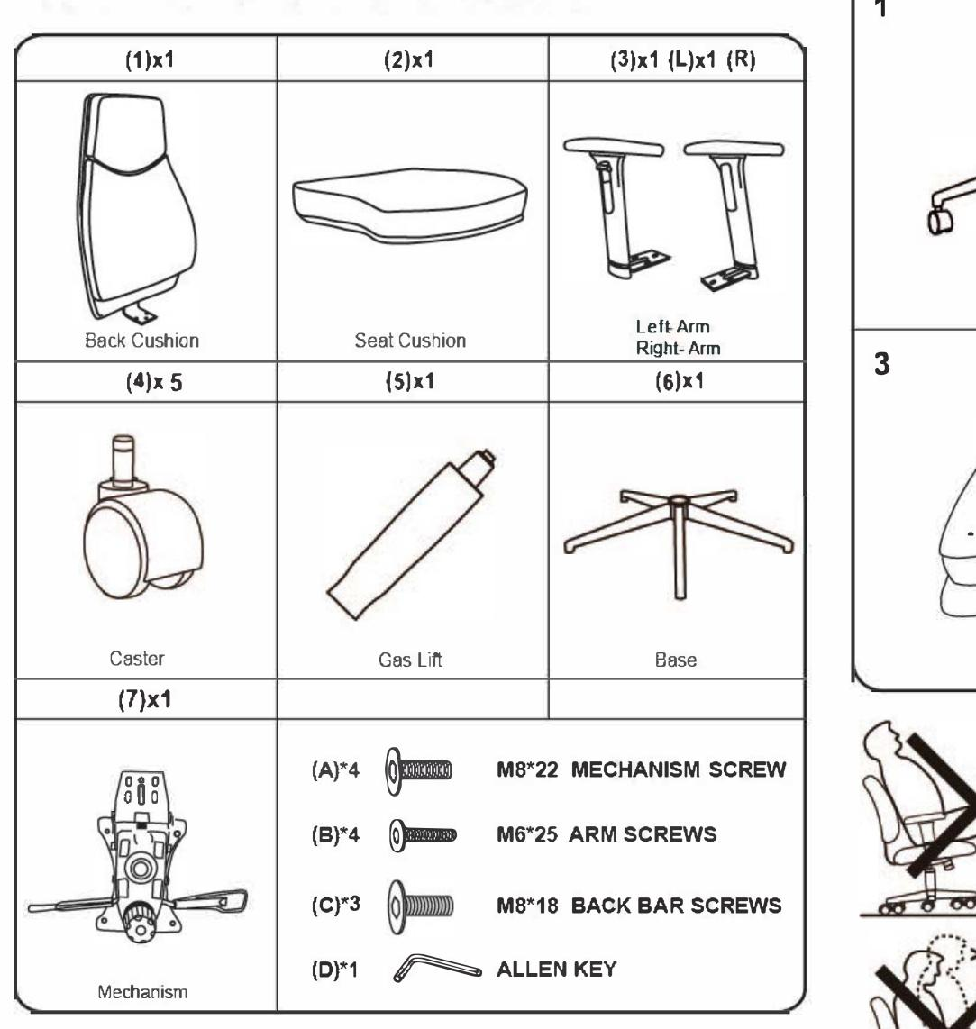
It is important to assemble all parts so that the directional "Arrows" point in the same direction. Make certain that all screws are FULLY tightened before using the chair. Each month, check all screws and tighten any that may have loosened.
