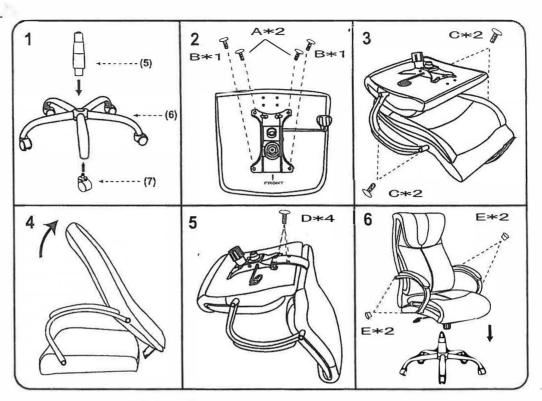
Note: Please tighten all arm screws using allen key before step 6
