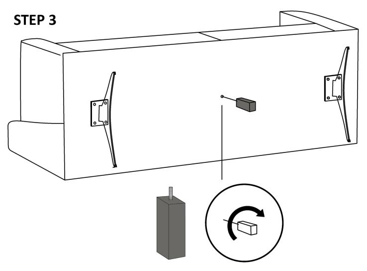
please find the fixing hole underneath, place the wooden leg and turn right
