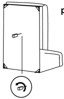
please find the fixing hole underneath, place the adjustable plastic leg
