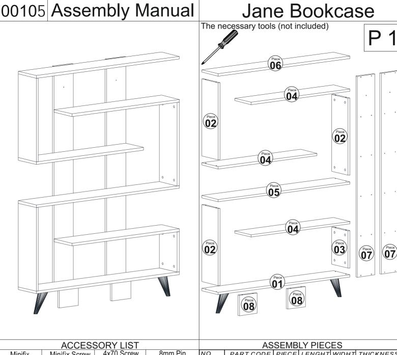
4x70 Screw 8mm Pin Minifix Minifix Screw NO PART CODE PIECE LENGHT WIDHT THICKNESS 00106.01 196 1200 18 2 00106.02 3 570 196 18 **20**x A02 2x A08 3 276 196 18 20x A45 00106.03 1 A01 4 3 900 196 18 00106.04 Retro Leg 3,5x18 Screw 4x50 Screw 5 1200 196 18 00106.05 1 6 00106.06 1200 196 18 White 7 00106.07 1488 160 18 A09 8x A04 20x 24x A46 8 150 160 00106.08
