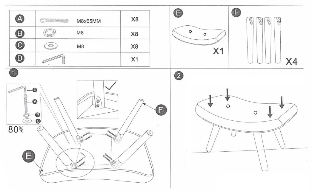
Pls do NOT fully-tighten all screws before adjusting the balance of the whole footrest
