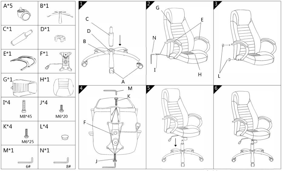
It is important to assemble all parts as the directional "Arrows" point to Make cerainthat all screws are FULLY tightened before using the chair. Each month check all screwsand tighten those that may have loosened.
